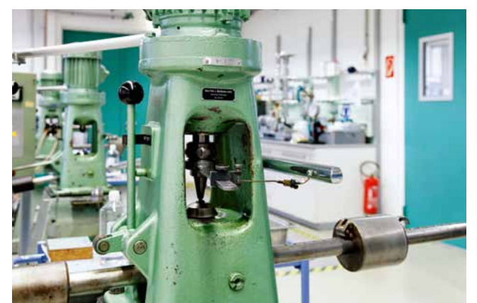
Four-ball tester | DIN 51350/1-6 The four-ball tester is used to assess lubricity under high pressure or wear. The set test force either causes the balls to weld together or the upper ball to leave wear scars on the lower balls. The welding force and the size of the wear scars are criteria for assessing the performance of a lubricant during development.
