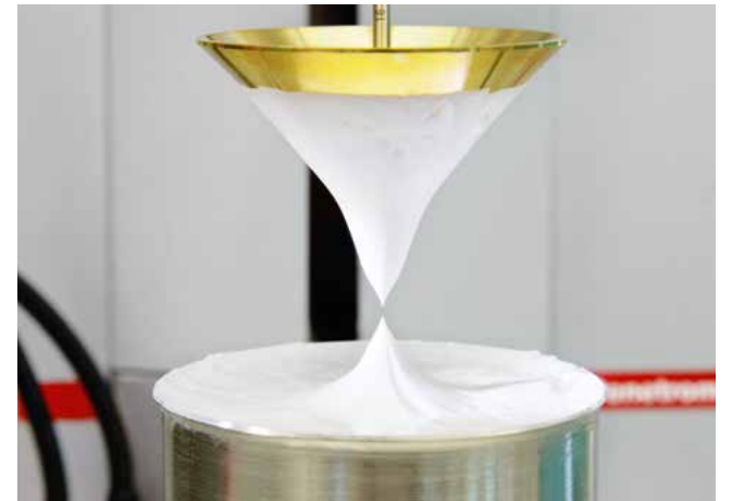
Penetrometer | DIN ISO 2137/ASTM D217 and ASTM D1403 The unworked penetration describes the penetration of a lubricating grease at 25 °C without previous mechanical wear stress. The higher the penetration depth of the test cone, the higher the penetration number, the softer the grease and the lower the consistency class according to NLGI.
