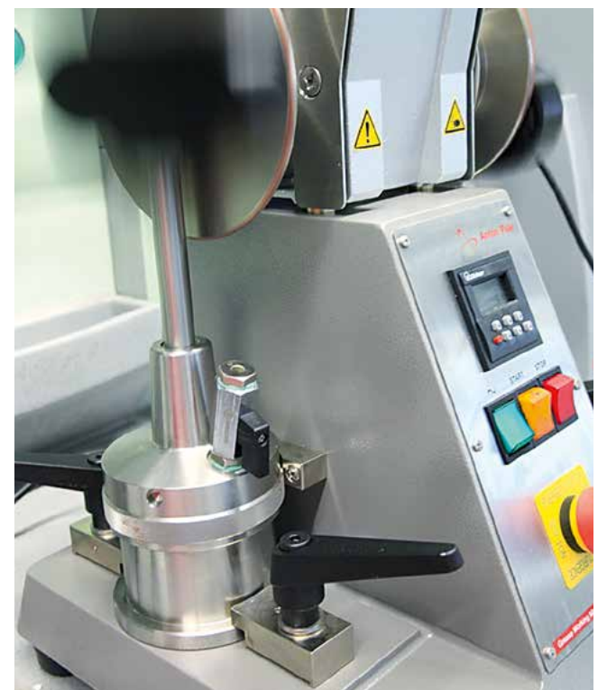
Grease worker | DIN ISO 2137 In the Grease Worker, the working penetration is determined regularly after 60 double cycles and the extended working penetration after 5,000 to 100,000 double cycles. The lower the deviation between unworked and worked penetration, the more stable the grease behaves during mechanical processing.
