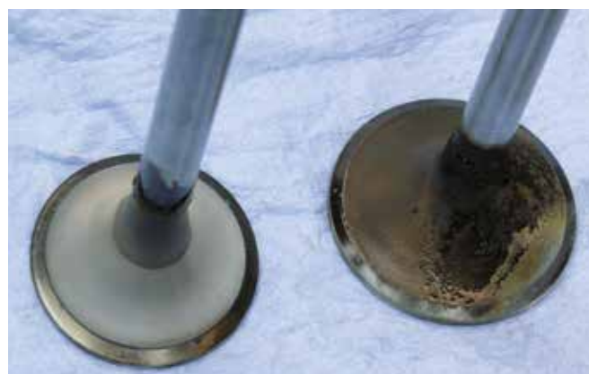
Inlet and exhaust valve – MTU Onsite Energy AB 3066 L4 V6
