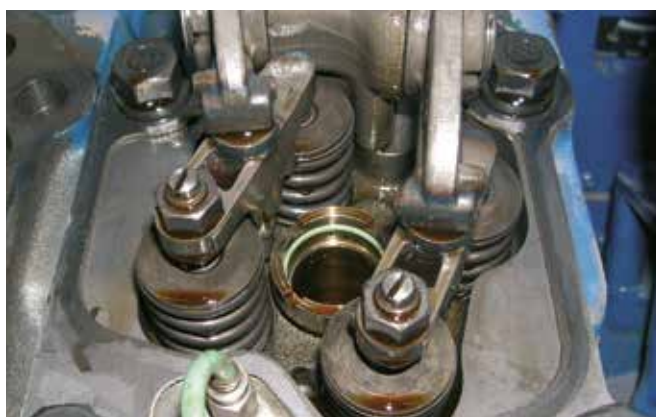
Valve train – MWM TCG 2016 V12
