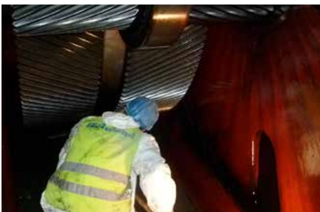
Gear unit inspection from inside
