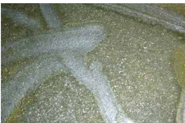
Deposit of metal chips on the gear unit housing floor
