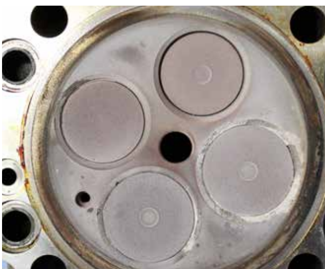
Field test engine MWM TCG 2016 V12 C, final diagnosis after 6000 operating hours – Cylinder head with valves (ignition area): Minimum deposits only without negative effects on valve sealing
