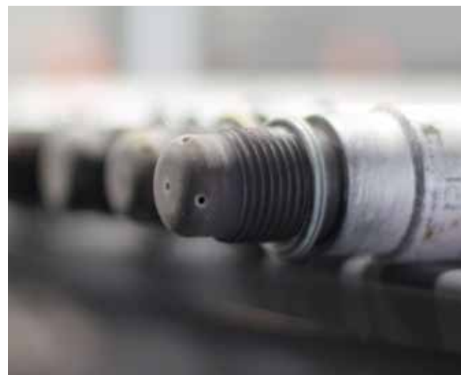
Field test engine MWM TCG 2016 V12 C, final diagnosis after 6000 operating hours – Spark plugs: Very clean, thus guaranteeing the best possible distribution of ignition sparks and thus optimal combustion of the gas mixture
