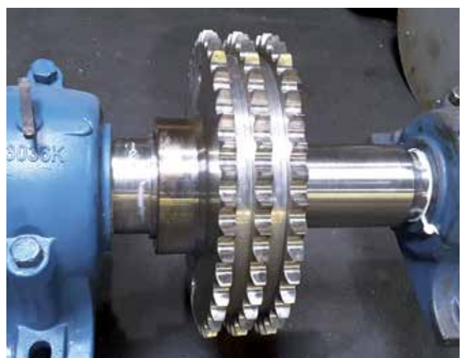
The Märkische Faser GmbH in Premnitz, Germany manufactures polyester fibres. In the plant nine roller works form a fibre train unit. Steam passes through quill shaft and rollers and heats the unit to temperatures up to about 180 °C. The bearings of this unit are exposed to high thermal and mechanical loads. These are ideal conditions for ADDIFLON PFPE Premium XH 2. The plants are running without any problems and the Märkische Faser GmbH as well as the responsible partner Öl & Filter in Trebbin are completely satisfied.
